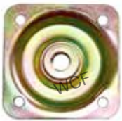
•771031 Leg Mounting Plate 45 x 45mm M8 Thread Yellow Zinc Plated
