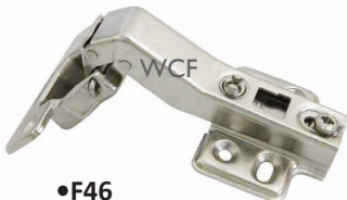
• F46 Hinge with Slide-on 4-Hole Plate 45° R4.95/R5.69 each
